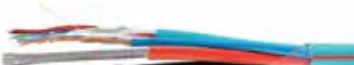
CREST-5: CREST-1 + 2x CAT5E 24 AWG UTP + 2 x RG6/U QUAD SHIELD, BUNDLED, PVC JKT
